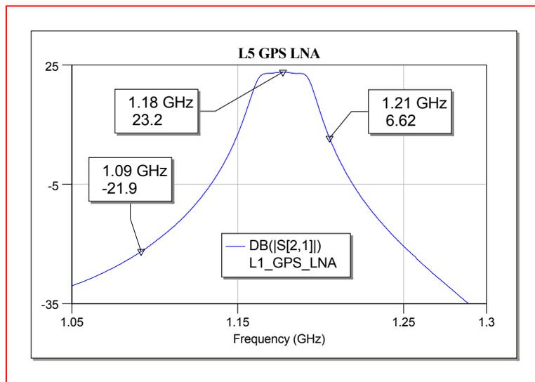
A 3-pole ceramic filter attenuates the transmitted RF pulse by 44 dB, reducing it to a level that is tolerable to a companion GPS receiver.
