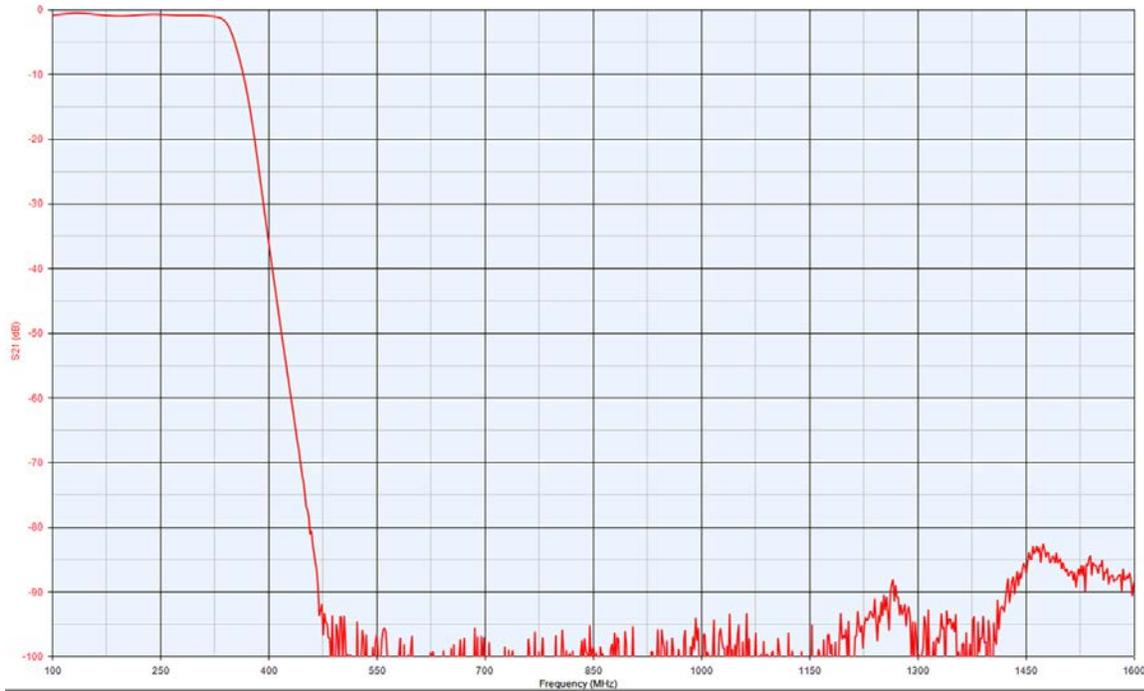
*Both a flat passband with low insertion loss and steep drop off on high power SFB filters is critical to enable the 100s of watts of RF power that are passed and filtered by these devices.*
