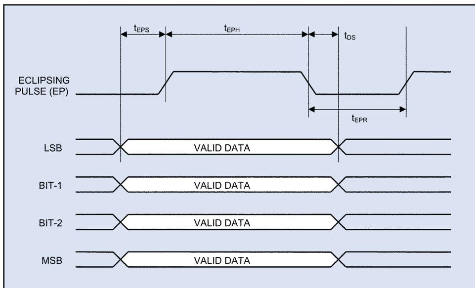
Fig. 3. Logic timing of the eclipsing pulse.
