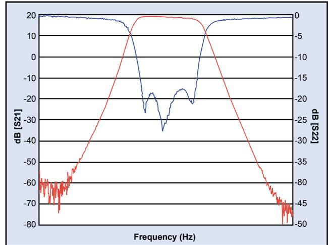
Fig. 4. The switch filter bank's typical transfer function and return loss.
